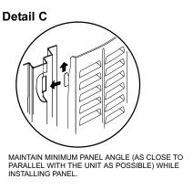
Figure 7. Removing and Installing Panels
